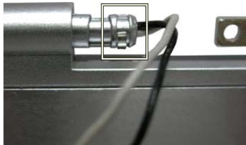
Fig. 23 Removing ring from right hinge
